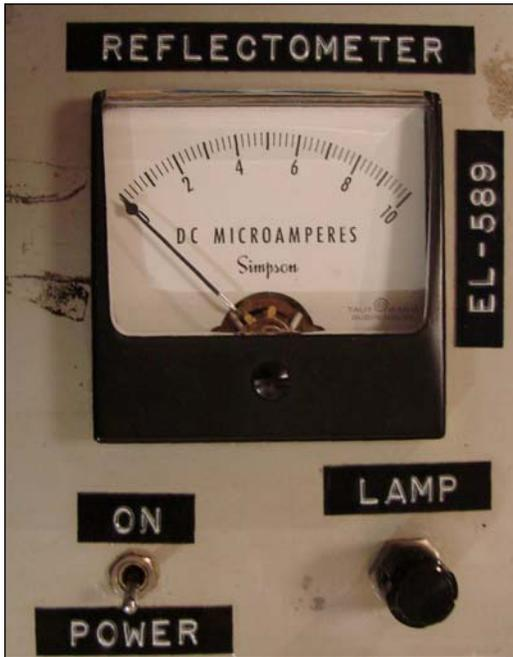
The instrument is quite simple to use. The electronics package has the power switch, lamp adjustment knob and meter.
