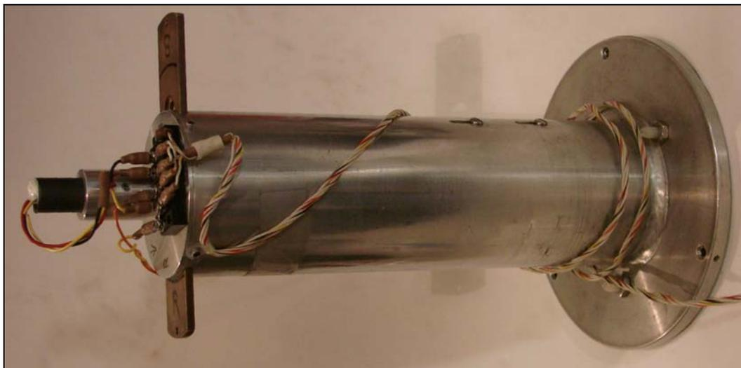
This is the sensor unit that is placed on the optic for testing. It has three small nylon feet that rest on the optic surface. These plastic feet help to reduce damage to the coating and optic. When placing the sensor use straight up and down motions only. Never slide the sensor on the optic surface as this would result in significant damage to the optic.
