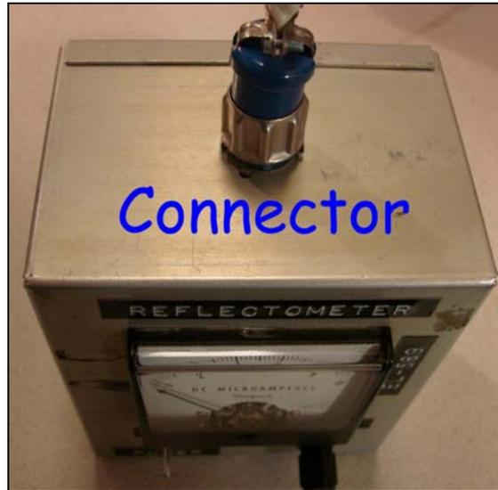
The sensor unit plugs into the top of the electronics box and the plug retainer is then locked into place to insure a good connection and the plug won't fall out and drag across the optic being tested.
